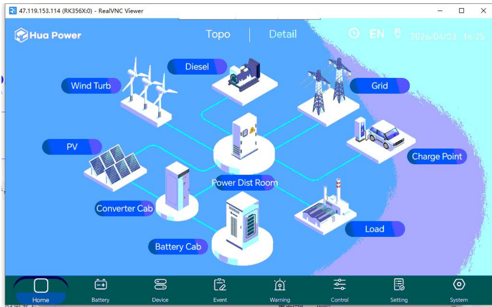
Figure 3-7 Schematic diagram of LC (Lightweight EMS )
