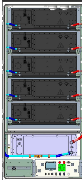
Figure 3-5: Battery Cluster Appearance
